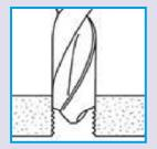
Drill out old threads with a standard drill. Note: Drill is oversize - see charts for proper dimensions. Chamfer the hole with a standard countersink (820-1000)
